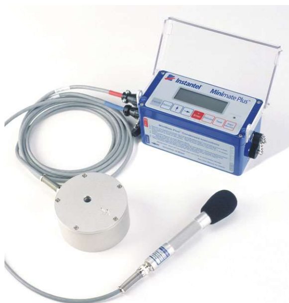
Figura 29: Sistema Minimate Plus da InstanTEL (InstanTEL, 2014)
